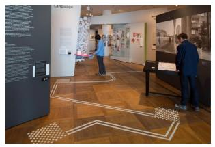
Figure 17: Tactile control system
